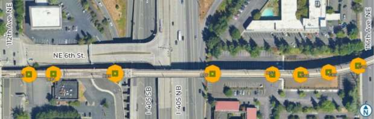
Figure 36: No Build Zone around Existing Drilled Shafts (background image credit: Google Maps).
