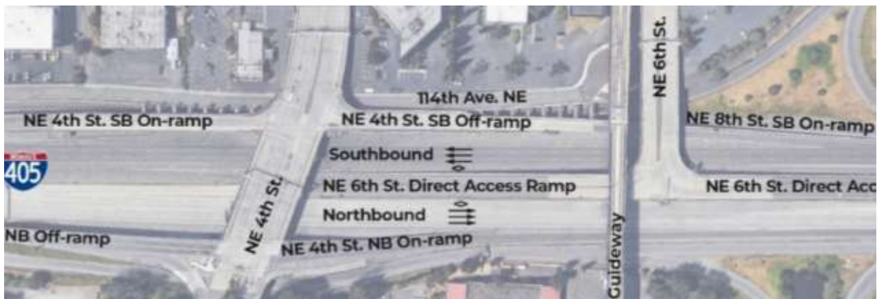
Figure 23: Current I-405 lane configuration within the project limits (background image credit: Google Maps).
