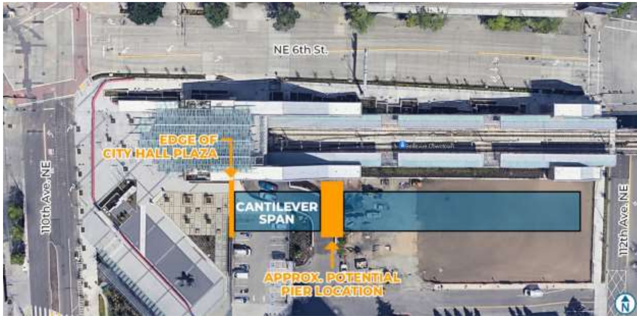
Figure 19: West tie-in schematic layout showing geometric constraints, plan view (background image credit: Google Maps).
