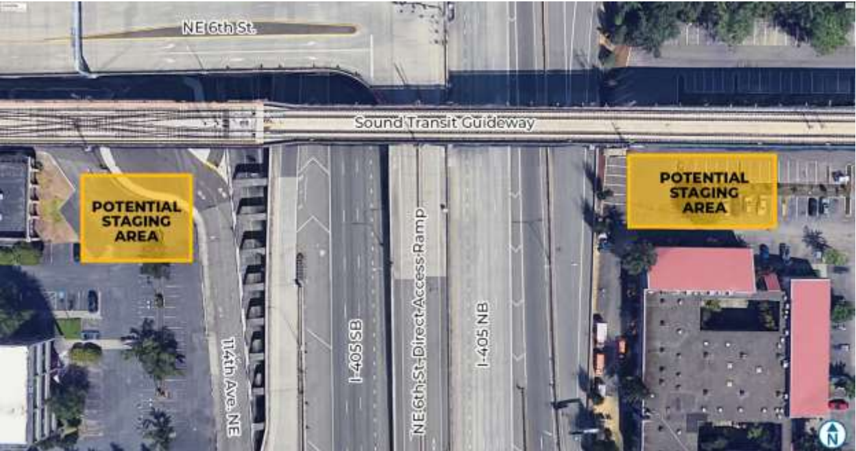
Figure 63: Potential staging area for I-405 crossing structure construction (photo credit to Google Earth).
