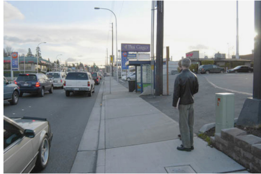
This photograph of the multiple curb cuts on a portion of Factoria Boulevard, north of SE 38th Street, illustrates the dominance of the automobile. The diagram at right suggests multiple businesses consolidating curb cut access points (red) and installing pedestrian connections (blue) between the three businesses and the sidewalk.
