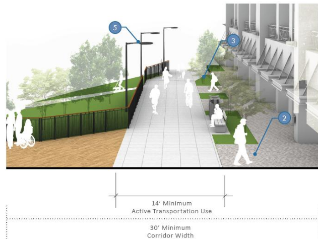
ACTIVE TRANSPORTATION ACCESS SECTION VIEW: CONDITION A
