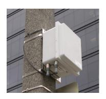
Bluetooth travel time collection hardware will be installed at four locations on Main Street.
