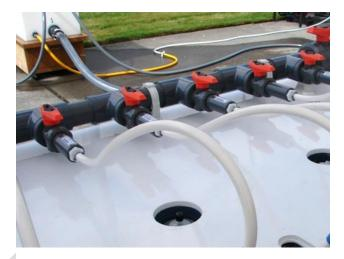
Piped Manifold Connected to Portable Blivet
