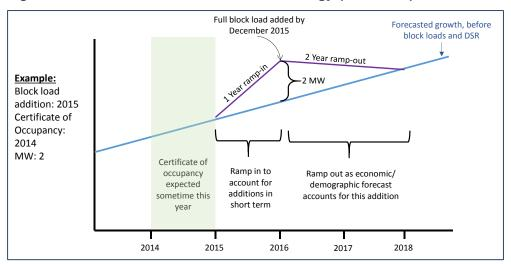
Figure 6.16: Block Load Addition Methodology (from PSE)
