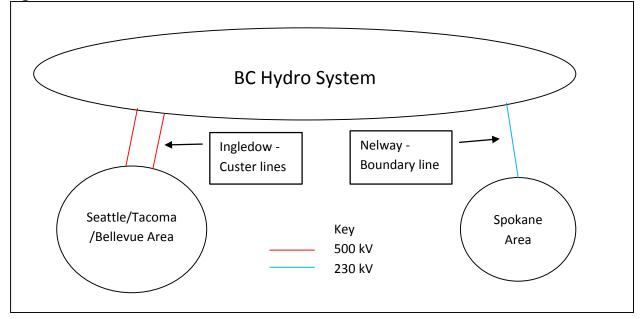
It should be noted when discussing Path 3 that sometimes the Nelway - Boundary 230 kV line is referred to as the Path 3 eastside intertie. This term should not be confused with eastside as it is used in the context of the Energize Eastside project. The Path 3 eastside intertie is located near Spokane, WA and is over 250 miles away from the area under consideration for the Energize Eastside project.
