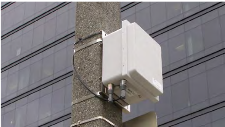
Figure 24. BlueTOAD Travel Time Unit on a street light pole
