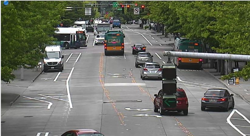
6 Vehicle loading/unloading in the bike lane before vertical separation was added to the painted buffer
