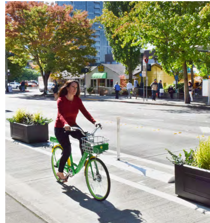
Figure 7. A person riding northbound in the bike lane north of NE 6th St, where curbs, posts, and planter boxes physically separate people on bikes from motor vehicle traffic.
