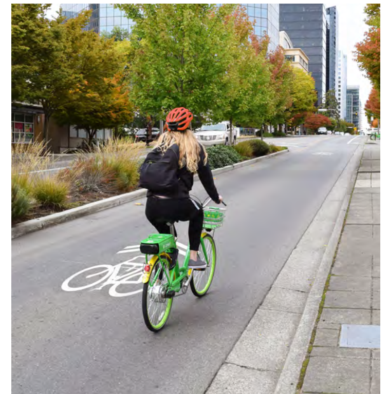
Figure 10. A person riding northbound in the marked shared lane north of Main St, where the travel lane is too narrow for a bike lane due to an existing planted median.
