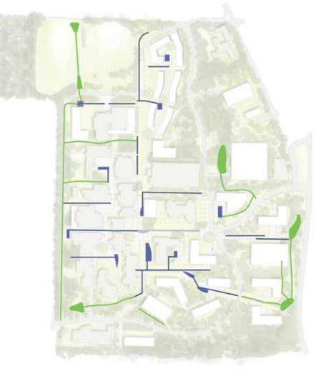
A campus-wide condenser water system will result in higher energy efficiency. The goal is to connect all buildings mechanically, providing the campus an ability to transfer energy where it's needed.
